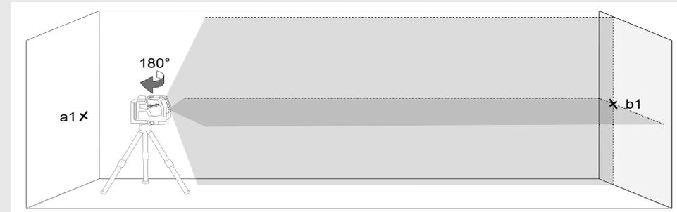
6. Move the laser level towards wall B and position it approximately 0.5 meter from wall B.
