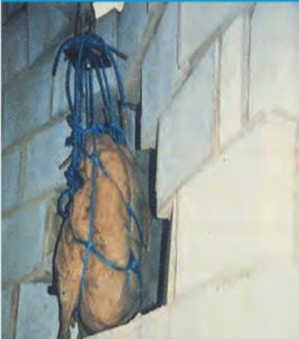
The picture right shows a Promat DURASTEEL® wall undergoing impact following a fire test. The picture above shows a concrete block wall undergoing similar testing.
