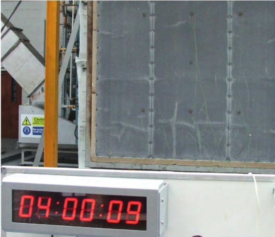
The picture above shows a Promat DURASTEEL® wall being fire tested to E240. Below are examples of Promat DURASTEEL® UK and International certification.
