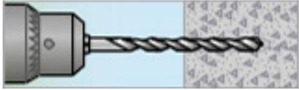
1. Drill an 8 mm hole. Depth minimum 30 mm.
