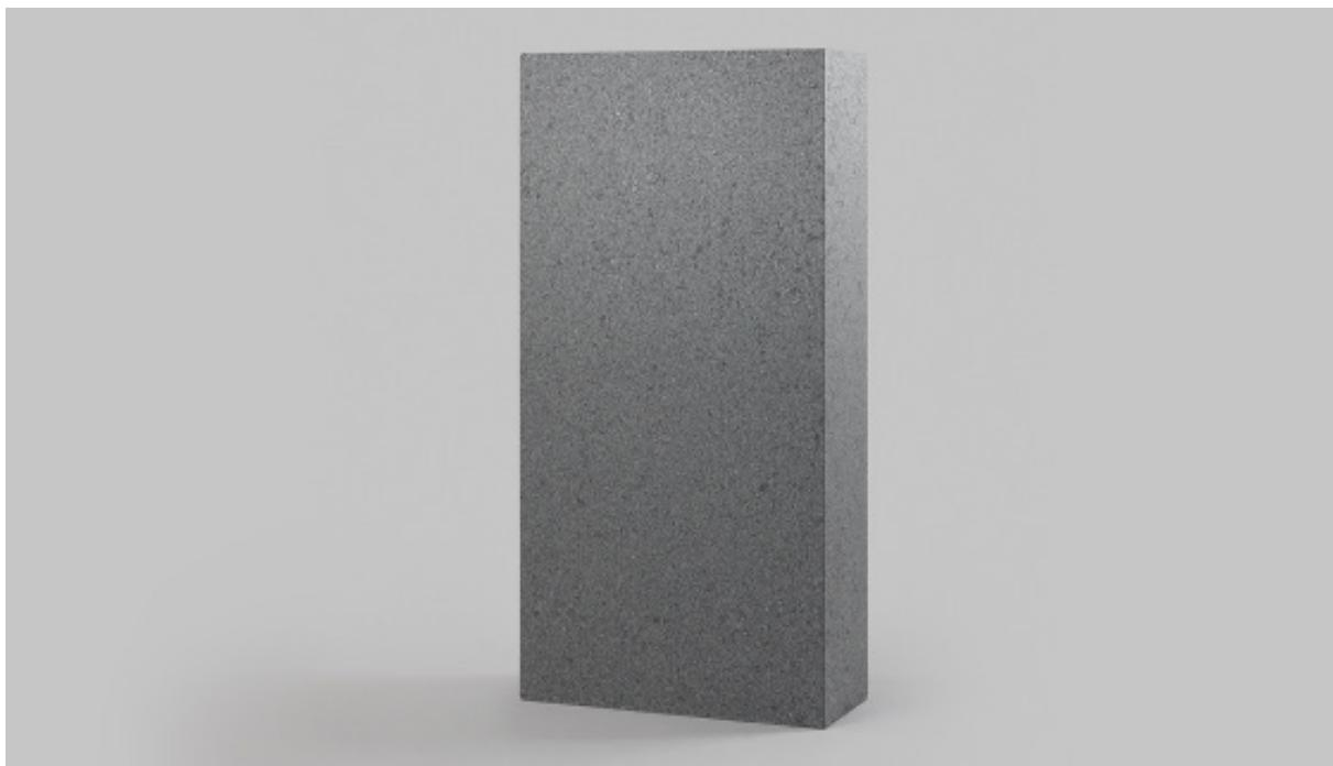
Sundolitt Climate C80 is a highly effective heat insulation material made of expanded polystyrene with addition of graphite. It's used as heat insulation in foundations, prefabricated concrete walls and combination roofs. The added graphite reflects and absorbs infrared heat radiation, which means that Climate C80 reduces heat loss by up to 25% compared to white EPS.
