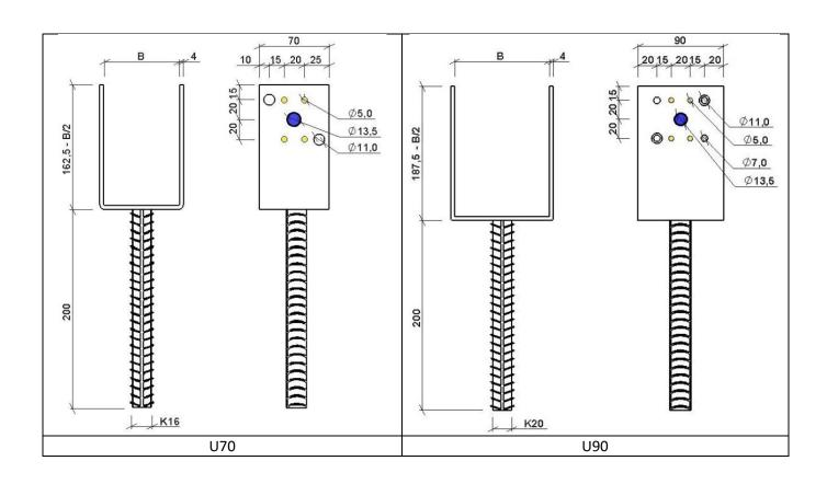
Load Capacity of U70 & U90 in C24-timber (350 kg/m³) with 8x 5x40 mm Anchor Screws
