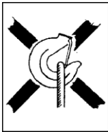
Fig 2 a The sling is applying load to the hook tip
