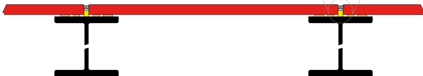
BALCONY FLOOR PANEL WITH SECRET FIXING (GLUED) ON STEEL BEAM
