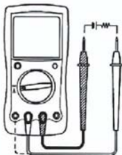
Fig 2. Current measurement DC
