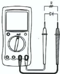
Fig 3. Resistance measurement Diode test Continuity test
