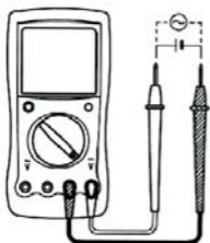
Fig 1. Voltage measurement DC and AC
