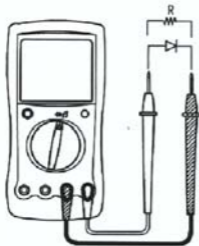
Fig 3. Resistance measurement Diode test Continuity test
